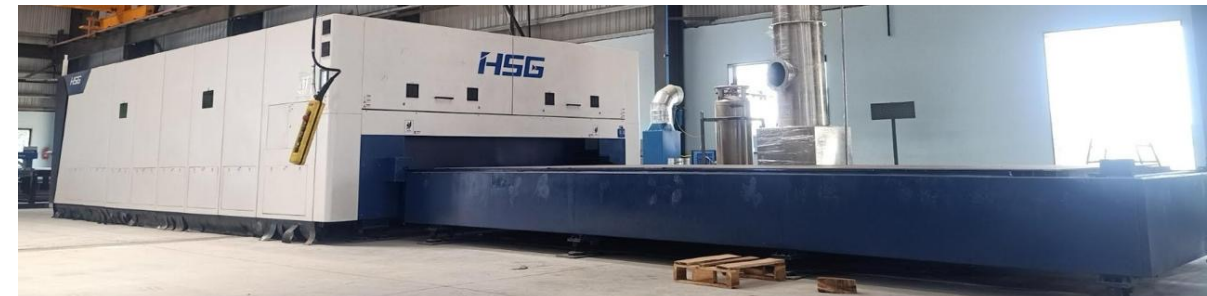
Laser cutting machine: 3 m x 12 m x 12 kw (August 2024)
