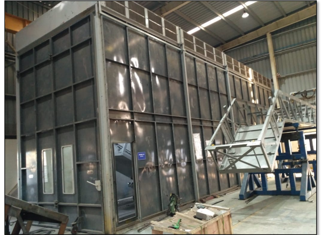
Down Draft Paint Booth SIZE :- 15.5 Mtr X 4 Mtr X 5.5 Mtr Height
